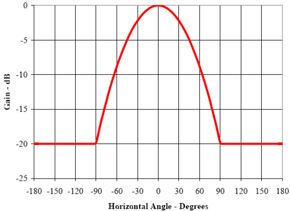
12 13 14 15 Figure 2: Antenna pattern for 3-sector cells
