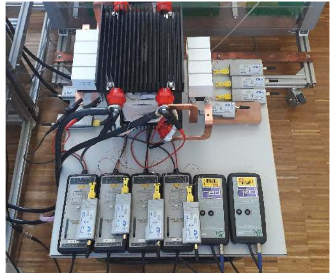
Fig. 15. MFT equipped with thermocouple probes for hot-spot temperature measurement
