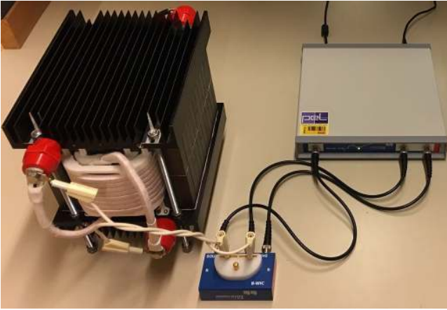
Fig. 10. Measurement of the electric parameters of the MFT
