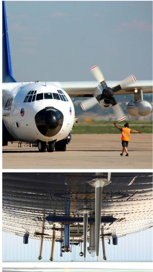
FIG. 2-6. (top) The NSF/NCAR C130 research aircraft with (bottom) multiple sampling inlets on the bottom of the fuselage. Photos by Sam Hall, UCAR.
