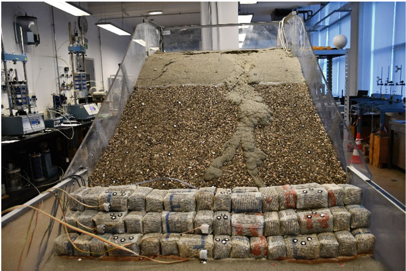
Fig. 6 Photo of small-scale model of a slope supported by gabion gravity wall exposed to impact of prolonged artificial rainfall
