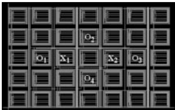
Fig. 11. Common centroid capacitor layout for the switch cap integrator.
