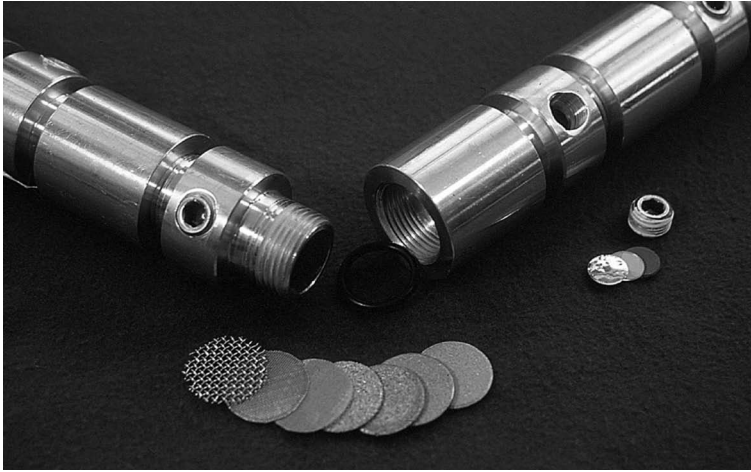
Figure 7. Integrating Diffusion Battery showing the porous plate collectors and the inserts used to hold collectors and track etch discs for detecting alpha particles emitted from the deposited particles. The unit may be assembled with as many sections as desired.
