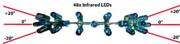
Fig. 4. Side view of the RABIT sensor showing the placement of the three 360^\circ infrared LED rings, giving \pm 20^\circ vertical coverage, each line represents the centre of the LEDs radiated \pm 25^\circ beam
