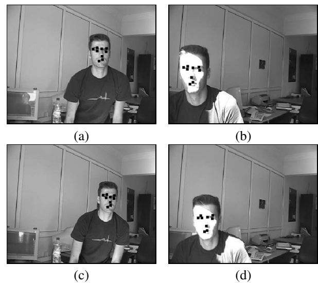
Fig. 17. Tracking results of the MF algorithm for a 450 frame segment of an indoor video sequence under varying lighting conditions. The existence of hard shadows on the face does not affect the tracking performance. The shown sample frames are taken at 150 frame intervals.
