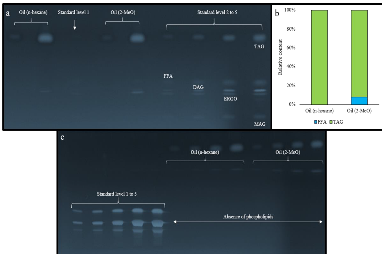
Fig. 1. a: HPTLC plate of neutral lipids; b: relative content of neutral lipids; c: HPTLC plate of polar lipids.
