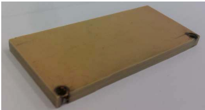
Fig. 6: Assembled passive substrate with embedded transformer
