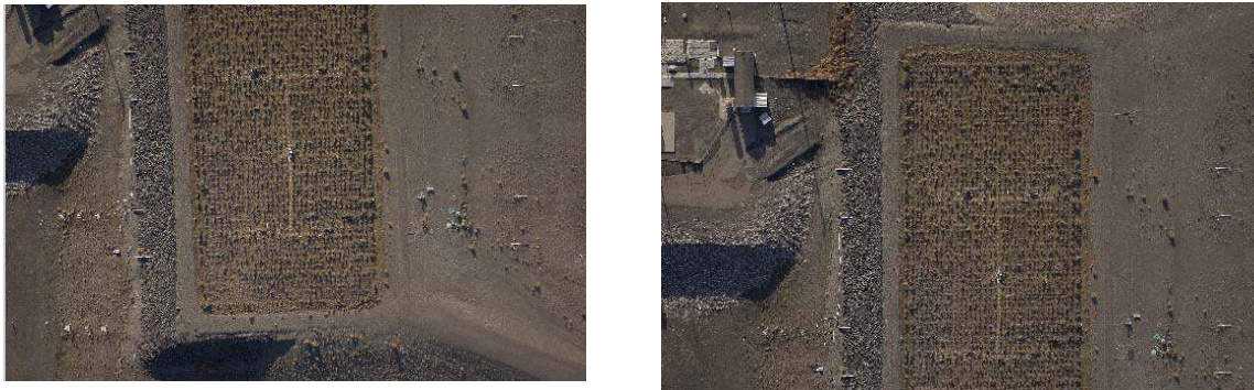
Figure 3.1. Example of two Overlapping Images used to Extract Control Point of Generation of the Digital Elevation Model
