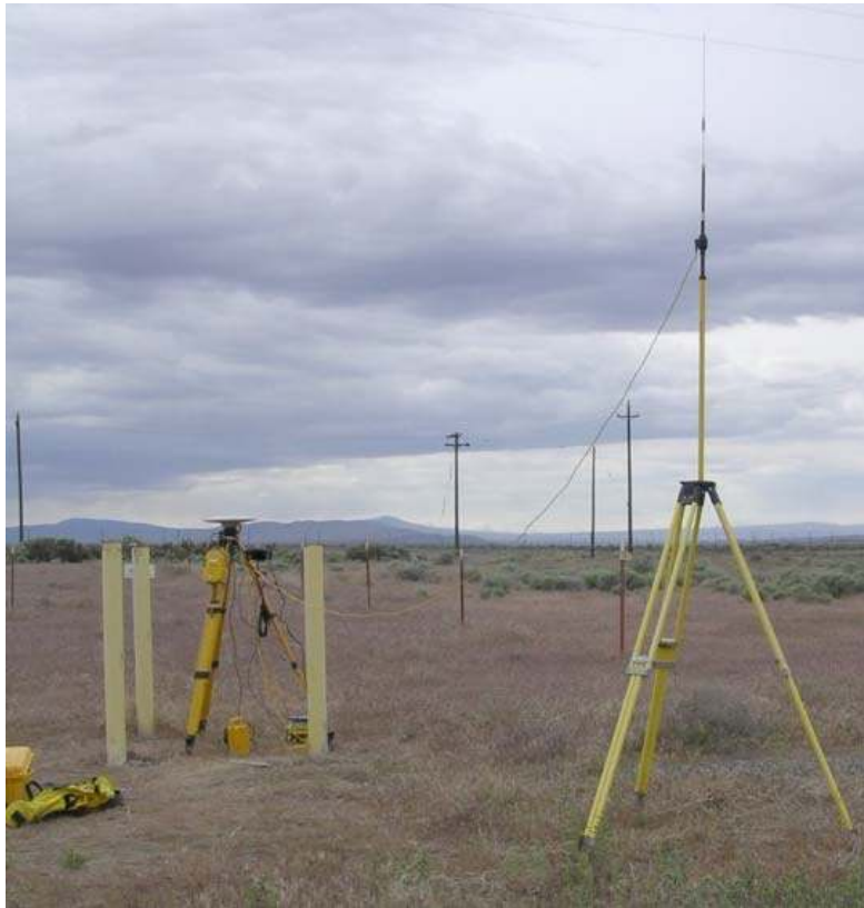
Figure 3.5. Real-Time Kinematic GPS Surveying System with a 5700 Receiver and Trimmark 3 Base Station Radio with Whip Antenna
