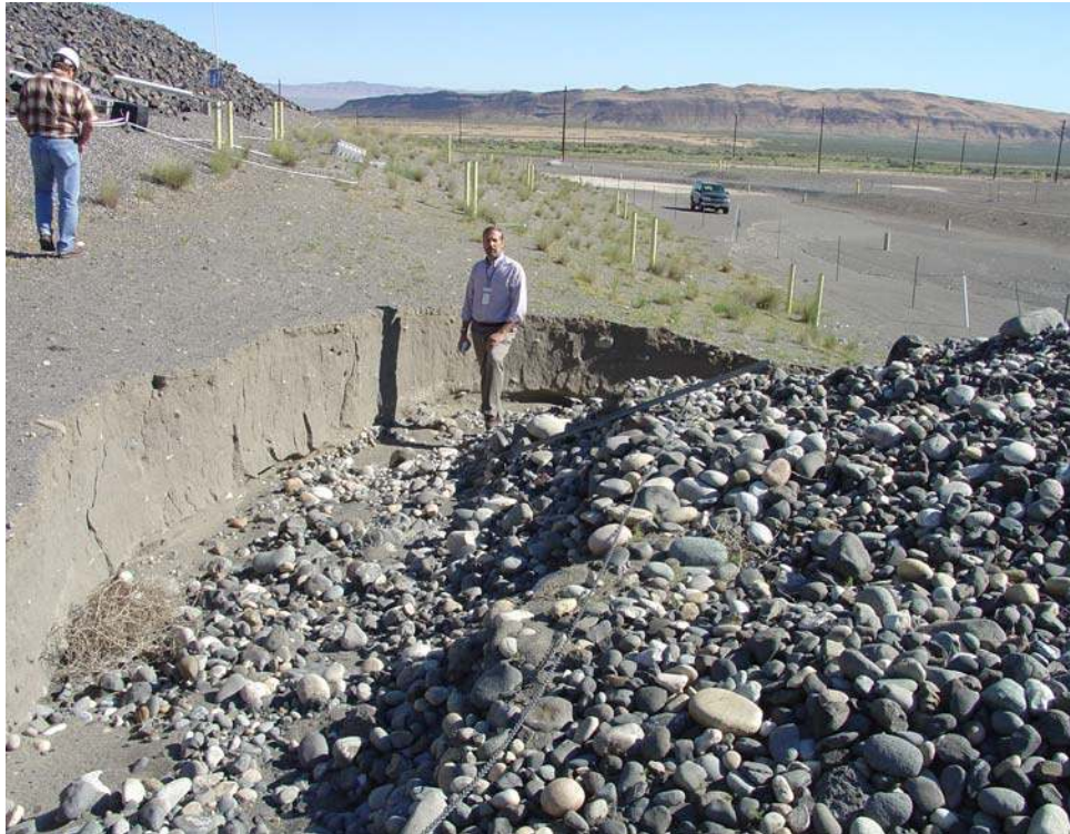
Figure 2.25. North-Facing Photograph Taken on 6/16/04 from the BY Tank Farm During an Inspection by Kirk Christensen and Curt Wittreich (standing in channel). The light colored area behind the vehicle is the fine-textured sediment remaining after the ponded runoff water infiltrated and evaporated adjacent to the BY Cribs.
