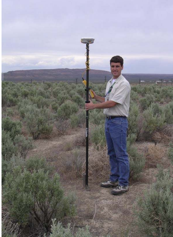
Figure 3.6. Real-Time Kinematic 5800 Rover Unit at the Prototype Barrier (Jason Keller supports the unit)
