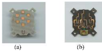
Fig. 5. Fabricated patch antenna (a) front and (b) back.
