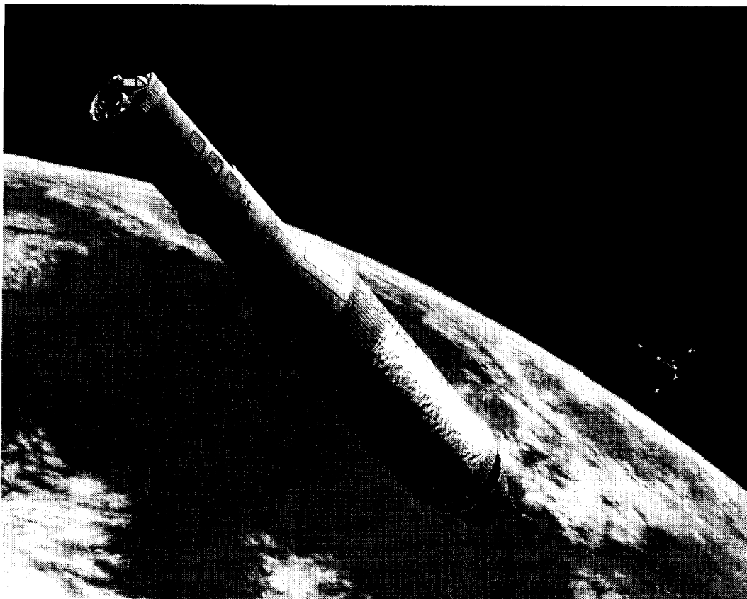
Figure 8.—A LANTR-powered Transfer Stage Leaves Earth Orbit Carrying a Passenger Transport Module on a "24 Hour" Trip to the Moon.
