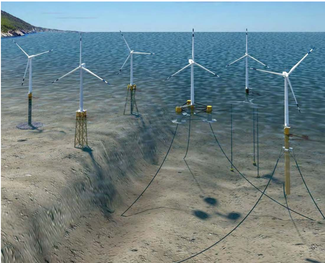
Figure 16. Offshore wind substructure designs for varying water depths. Illustration by Josh Bauer, NREL
