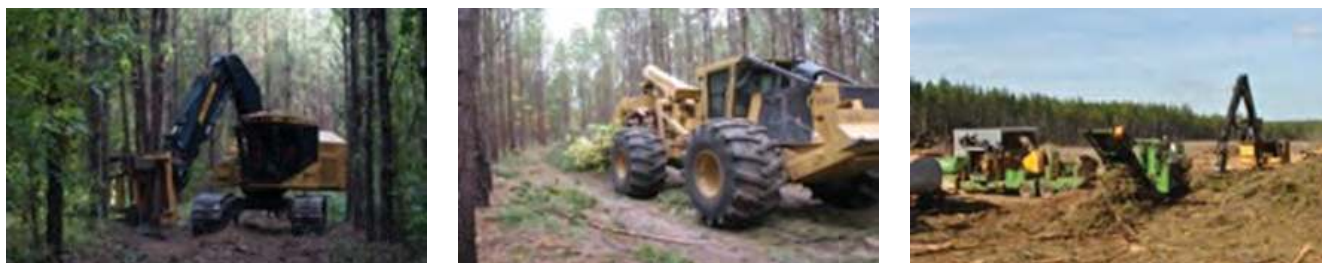
Figure 3.6 | Machines for harvesting trees and forest residues
