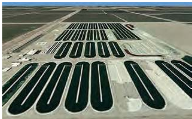
Figure 7.2 | Traditional open-pond raceway design used in the current analysis
