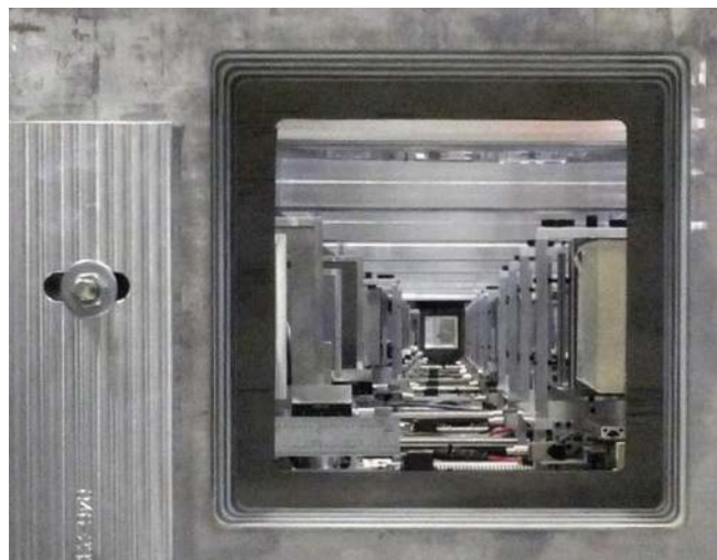
FIGURE 2: An upstream view through the vSANS guide boxes at NG-3.
