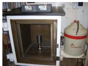
FIGURE 1: The second-generation detection system installed in the dedicated low-background counting room. The new Ge detector “Glen” is seen in the center of the shielding.
