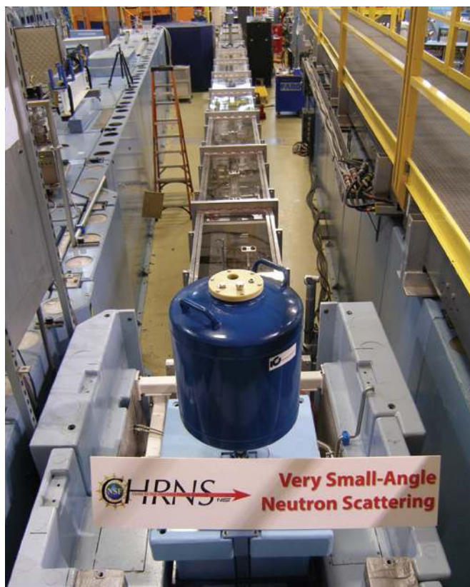
FIGURE 1: vSANS pre-sample flight path assembled and aligned.
