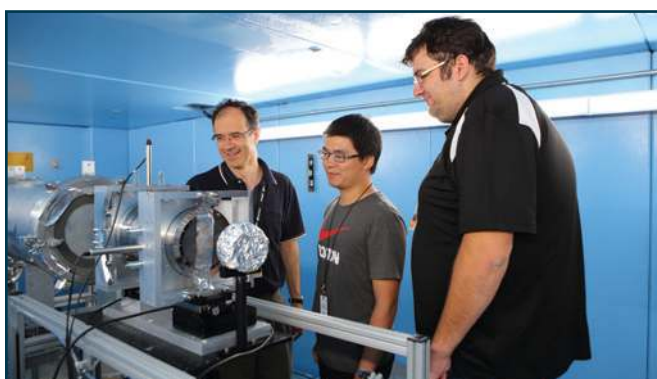
Boris Khaykovich and Huarui Wu from MIT, and Samuel Richardson (NASA summer intern) are characterizing their latest Wolter optics at the NG6 Cold Neutron Imaging Facility.
