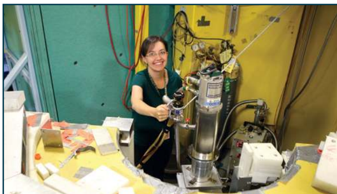
Amber Larson (U. Maryland) collects powder diffraction data from a Hollandite sample at BT1.
