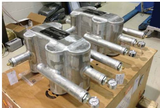
FIGURE 1: Deuterium condensers prior to enclosure in vacuum and helium containment jackets.
