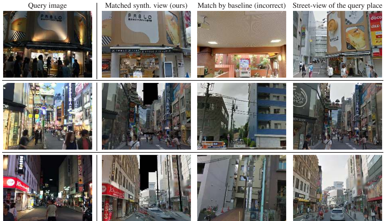
Figure 8. Example place recognition results for our method (Dense VLAD SYNTH) compared to baseline using only sparsely sampled feature points (Sparse FV). (Left) Query image. (2nd column) The best matching synthesized view by our method (correct). (3rd column) The best matching street-view image by the baseline (Sparse Fisher vectors without synthesized views). (4th column) The original street-view image at the closest position to the query. Note that our method can match difficult queries with challenging illumination conditions.
