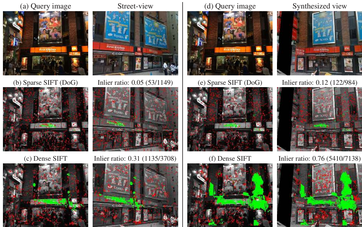
Figure 2. Matching across illumination and structural changes in the scene. First row: The same query image is matched to a street-view image depicting the same place from a different viewpoint (a) and to a synthesized virtual view depicting the query place from the same viewpoint (d). Second row: Matching sparsely sampled SIFT descriptors across a major change in illumination is difficult for the same (e) as well as for the different (b) viewpoints. Third row: Densely sampled descriptors can be matched across a large change in illumination (c) and the matching is much easier when the viewpoint is similar (f). In all cases the tentative matches are shown in red and geometrically verified matches are shown in green. Note how the proposed method (f), based on densely sampled descriptors coupled with virtual view synthesis, obtains significantly higher inlier ratio (0.76) on this challenging image pair with major illumination and structural changes in the scene.
