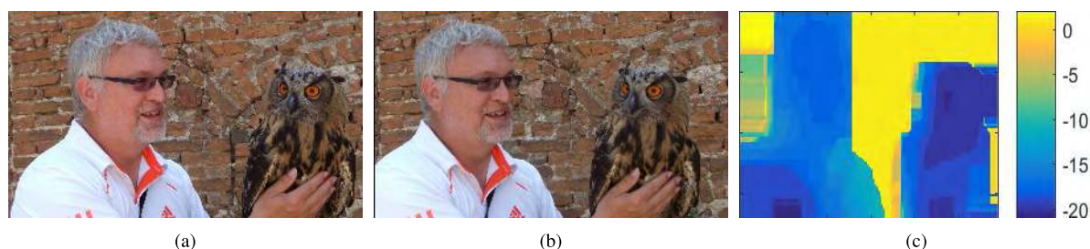
FIGURE 2. A distortion-free 3D image that has a low subjective quality owing to its non-positive disparity map and window violation problem at the left image boundary. (a) Left view. (b) Right view. (c) Horizontal disparity map.
