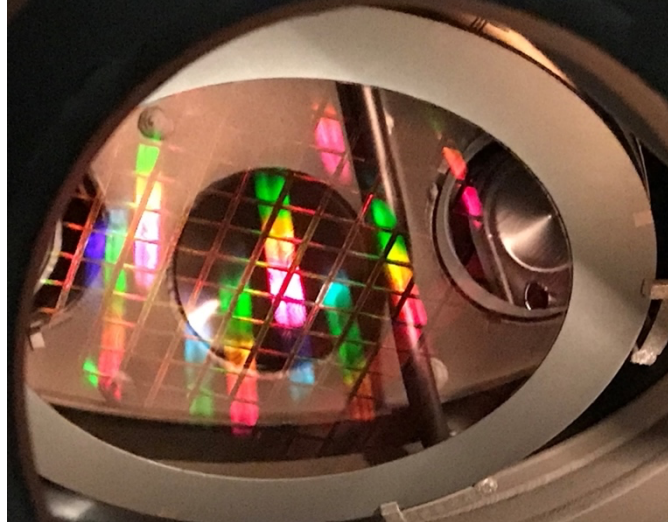
(7b) 200mm wafer with CMOS detectors in the MBE chamber
