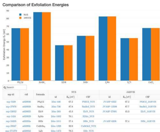
Fig. 2 Comparison of exfoliation energies from 2D MatPedia with NIST's JARVIS. A table in the interactive MPContribs landing page links each MP material to the according entries in the 2D MatPedia and JARVIS-DFT websites.
