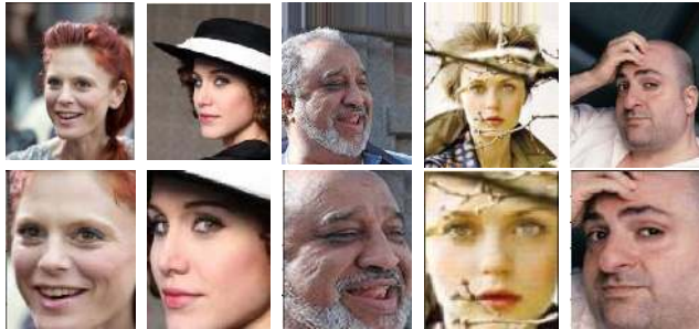
FIGURE 8. Examples of MTCNN for face detection (The top row is original images, the bottom row is cropped faces using MTCNN).
