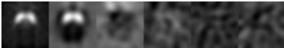
Figure 12: Images reconstructed from the first six KL components of the data (see Fig. 10). All but the first three are dominated by noise and can be omitted from the computations.
