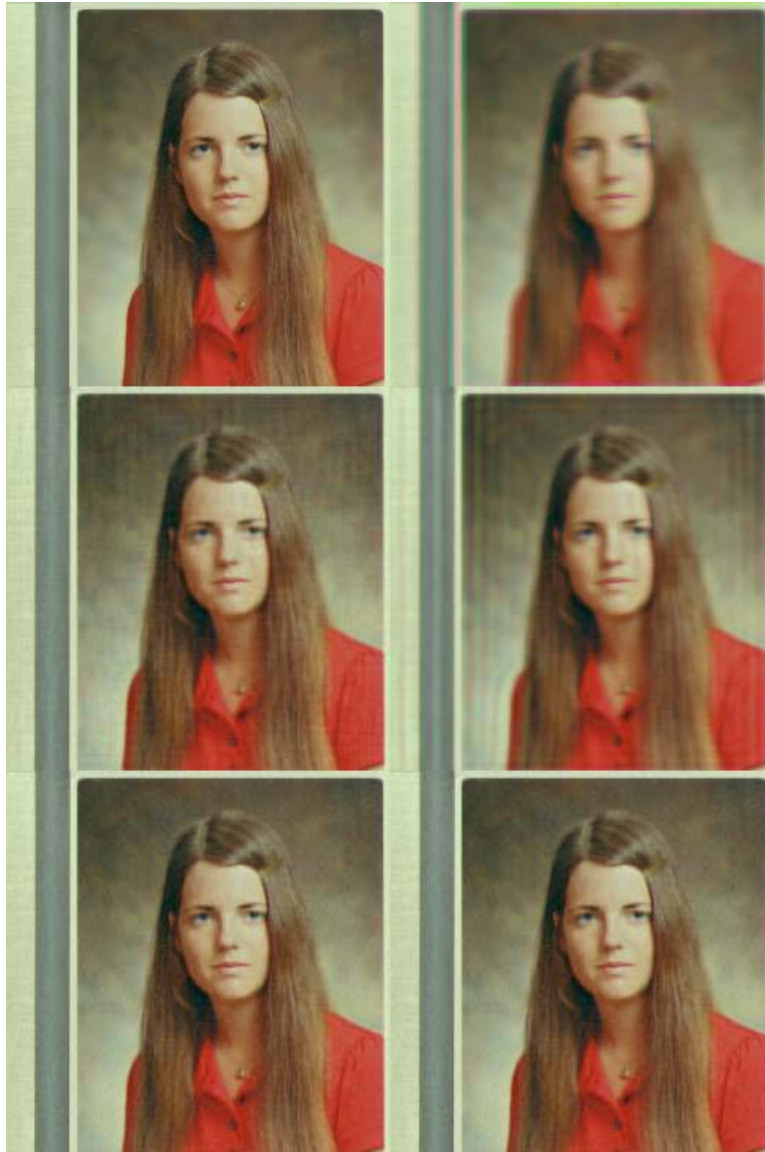
Figure 2: Example of a multichannel LMMSE restoration, original (upper left), degraded (upper right), restored single-channel power-spectrum from original (middle left), restored single-channel power-spectrum from degraded original (middle right), restored multi-channel power-spectrum from original (lower left), restored multi-channel power-spectrum from degraded (lower right).
