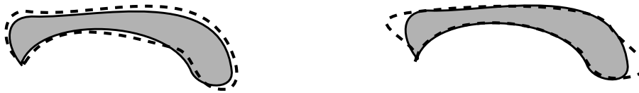
Figure 43: A scenario that demands more discriminative evaluation. The shaded region is the ground truth segmentation given by an expert, and dashed outlines are results yielded by the registration algorithm. Suppose the two examples have the same number of mislabelled voxels, using the ratio of mislabelled voxels will give them the same evaluation. However, in terms of segmentation quality, the example shown on the left is better than the one shown on the right.
