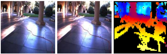
Figure 12: Two images taken from a stereo pair of cameras, and the depthmap calculated by a stereo system.
