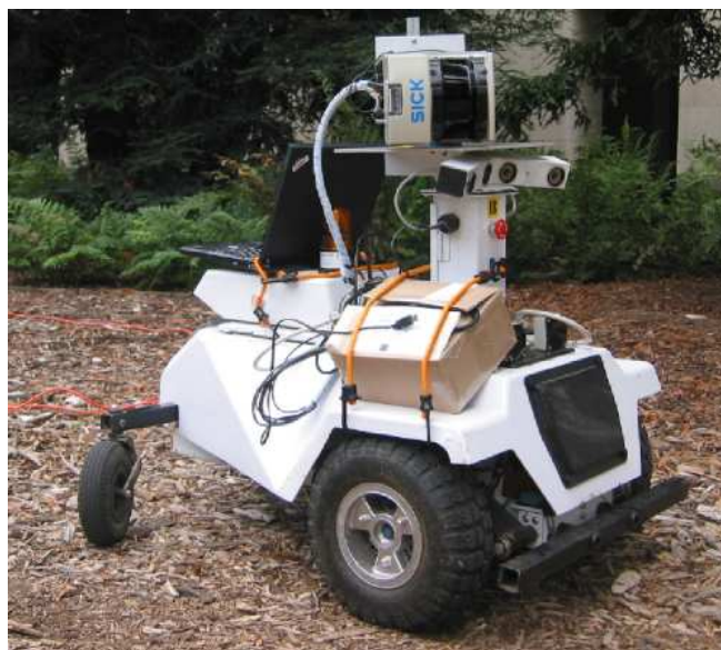
Figure 8: The custom built 3-d scanner for collecting depthmaps with stereo image pairs, mounted on the LAGR robot.
