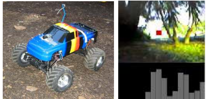
Figure 11: (a) The remote-controlled car driven autonomously in various cluttered unconstrained environments, using our algorithm. (b) A view from the car, with the chosen steering direction indicated by the red square; the estimated distances to obstacles in the different directions are shown by the bar graph below the image.
