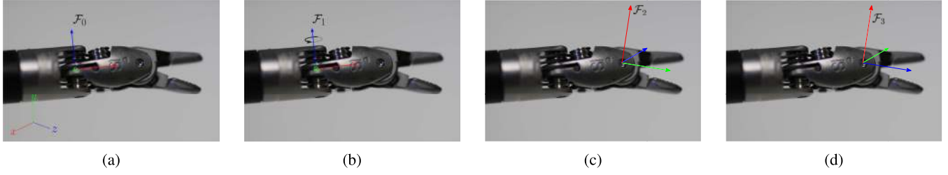
Fig. 5. (a) The base frame \mathcal{F}_0 for the robotic instrument which is oriented relative to the surgical camera with the rigid body transform {}^c\mathbf{T}_m . (b) The wrist frame \mathcal{F}_1 , which enables the instrument head to rotate around the z axis of this frame. (c) The claspers rotate together around the z axis of \mathcal{F}_1 defining a new frame \mathcal{F}_2 which has its x axis pointing in the direction of the claspers. (d) The claspers rotate around the z axis of this frame in opposite directions allowing opening and closing.
