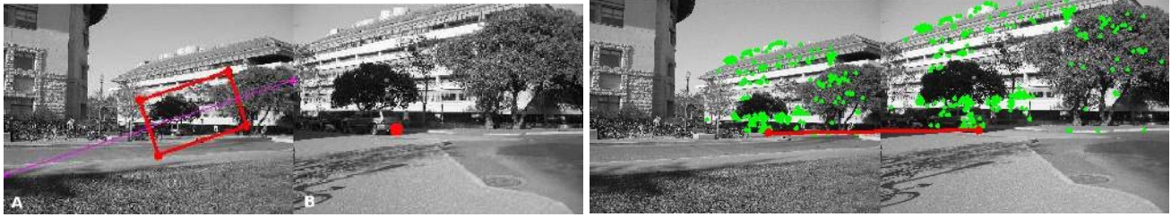
Figure 7. (a) Corresponding region to search for in image A, for a point in image B, (b) Correspondences found using our monocular depth estimates.
