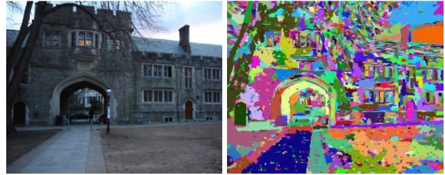
Figure 1. (a) An image of a scene. (c) Over-segmented image. Each small segment (superpixel) lies on a plane in the 3d scene.
