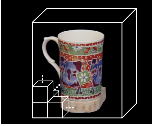
Figure 3: Bounding box of the volume with four voxels for illustration purposes.
