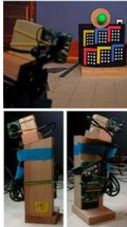
Fig. 7. To measure ground truth, we mounted board cameras taken out of webcams atop specially constructed stands, and set the stands and target on a flat, measured grid surface.
