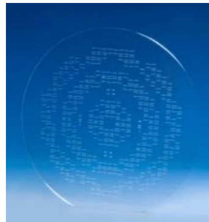
Figure 4: An example of a glass wafer with TGV using W-plugs (courtesy of Schott)
