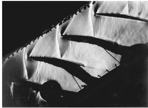
Fig. 2 Schlieren photo at M_1 = 1.09 , \beta_1 = 147.1 deg
