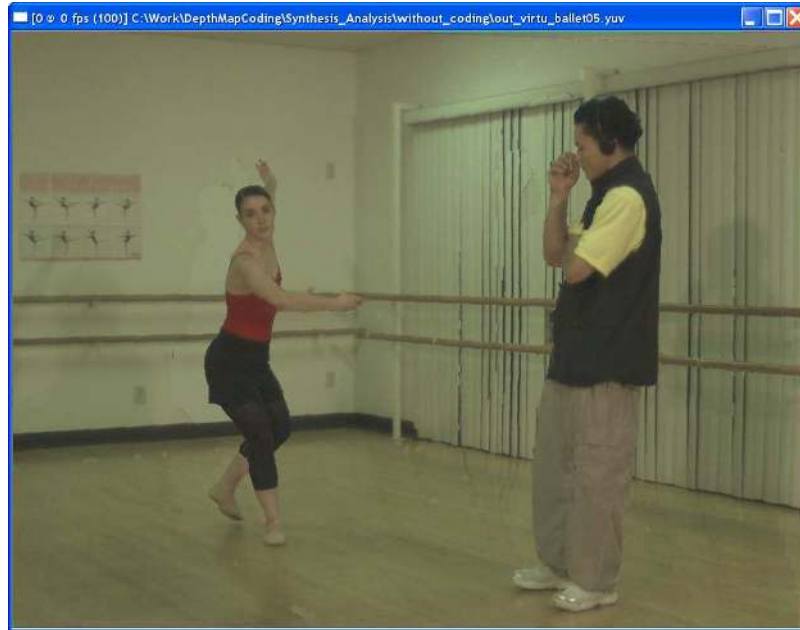
Figure 2.5: Subjective quality comparison of Ballet sequence; Synthesized 5th view without coding reference views. This results in 33.2 dB (Y PSNR).
