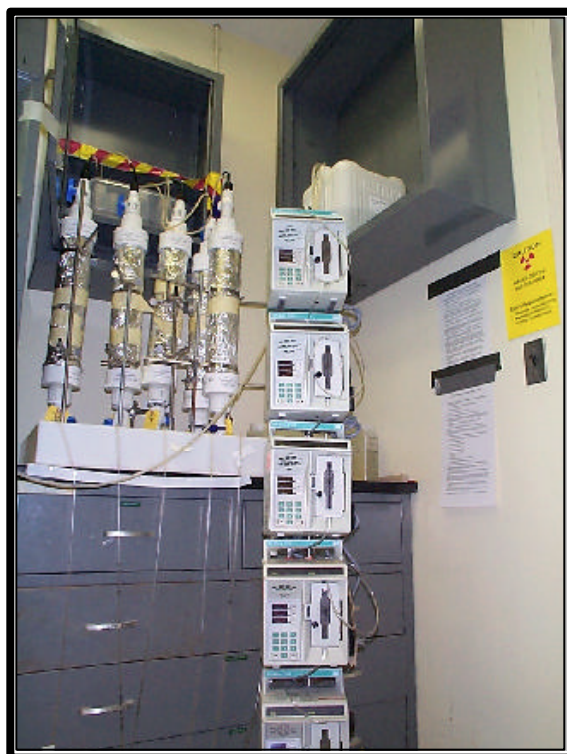
Figure 3.1 Flow-Through Column Leach Test
