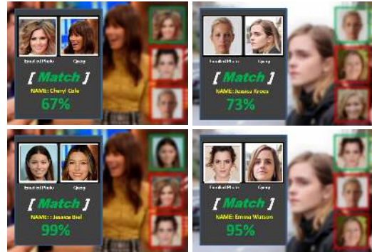
Figure 1: Face recognition with large pose variations. Top: Traditional face recognition system fails due to large pose variations. Bottom: The proposed 3D-PIM recovers natural frontal face images from arbitrary poses and recognizes the face correctly. Moreover, our 3D-PIM model potentially benefits face attribute recognition. Best viewed in color.
