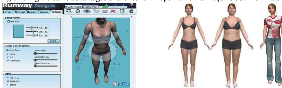
Fig. 21. Left: fully parametrized virtual human body model used in virtual-try-on application, Runway 3D of OptiTex Ltd. (Israel). Right: virtual anthropometric mannequins based on anthropometric data, from IFTH (France).
