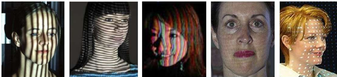
Fig. 7. Examples of projected light pattern. From left to right: vertical stripes by 3D-Shape GmbH (Germany), horizontal lines by Wicks and Wilson Ltd. (UK), color coding by Sanyo Electric Co.Ltd. (Japan), squared pattern by Eyetronics NV (Belgium), dot pattern by VX Technologies Inc. (Canada).
