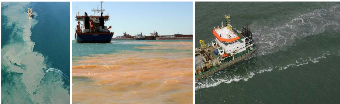
Figure 1.2: Two examples with and one example without visible surface overflow dredging plume (right photograph from H. Elbers Royal Boskalis Westminster).
