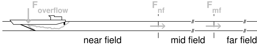
Figure 2.1: Schematic overview of the near field, mid field and far field of a dredging plume with the suspended sediment fluxes S_{j0} , S_{nf} , S_{mf} indicated.
