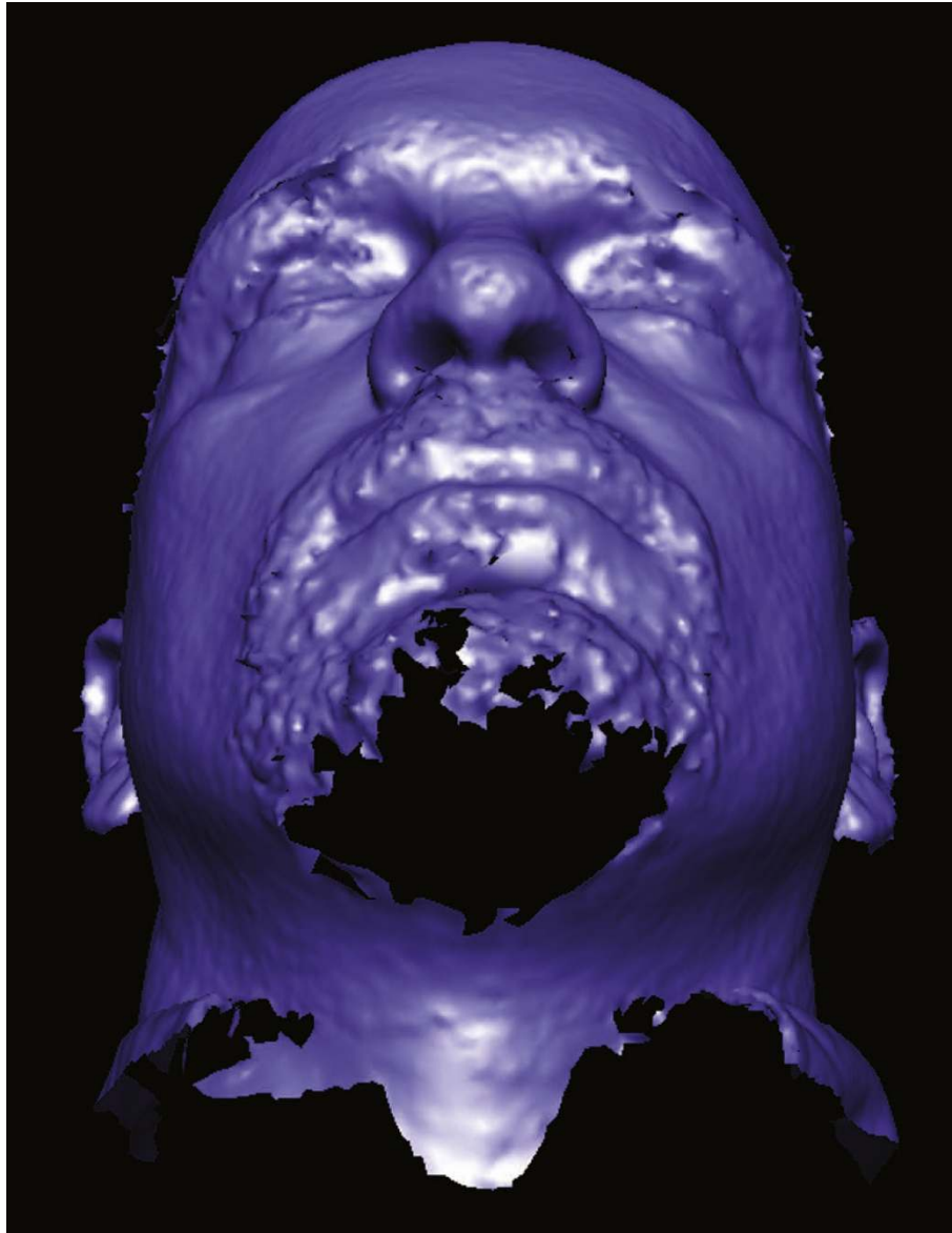
Figure 4 Surface data loss due to the presence of excess facial hair Color and texture information have been removed from this 3D model.
