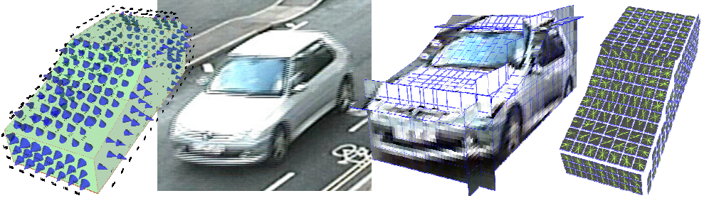
Figure 3 Extraction pipeline: 3D model with interest points \mathbf{P} followed by input image I , extracted image patches \mathbf{I}_p and feature vectors \hat{\mathbf{f}}_k . The radius of cones indicates the weight q_j of interest points \mathbf{p}_j . If a cone is missing from the grid, it was either not visible during training or gave poor performance and was rejected accordingly.
