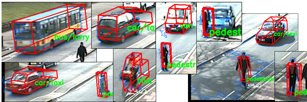
Figure 5 True positive examples for vehicles and pedestrians using 3DHOG.
