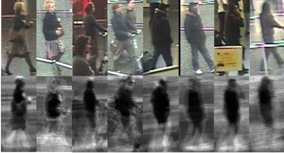
Figure 2: The top row represents example images sampled from person sequences of iLIDS-VID dataset, each 2 adjacent images represent a correct match. The bottom row includes the temporal gradient computed for these sequences and averaged over the frames involved.
