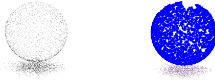
Fig. 5. Two tangent surfaces: (Left) The original point cloud. (Right) The two largest connected components: part of a sphere and part of a plane. The two components contain roughly 94% of the cloud.
