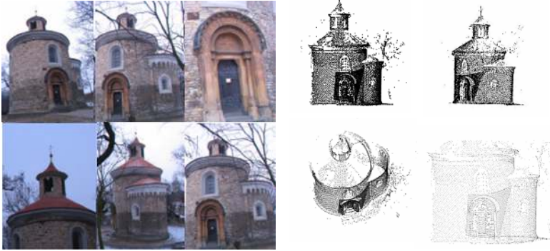
Fig. 3. The Data Pipeline: A series of images and the 3D cloud reconstructed from them. The area around the door is reconstructed at much higher density than the rest of the cloud.
