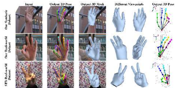
Figure 1: Our proposed method is able to not only estimate 2D/3D hand joint locations, but also recover a full 3D mesh of hand surface from a single RGB image. We show our estimation results on our proposed synthetic and real-world datasets as well as the STB real-world dataset [62].
