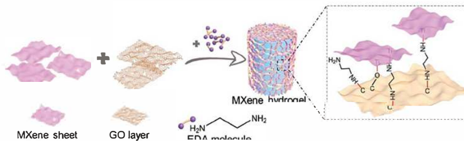
Figure 1. Schematic illustration of the formation process of MXene hydrogel.
