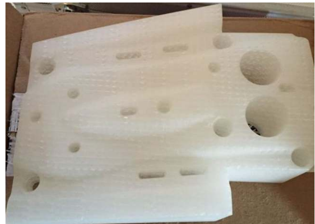
Fig. 16: Casting pattern for the trim pad shown in Fig. 10. This casting pattern was 3D-printed with SLA QuickCast technology using CastPro™ resin
