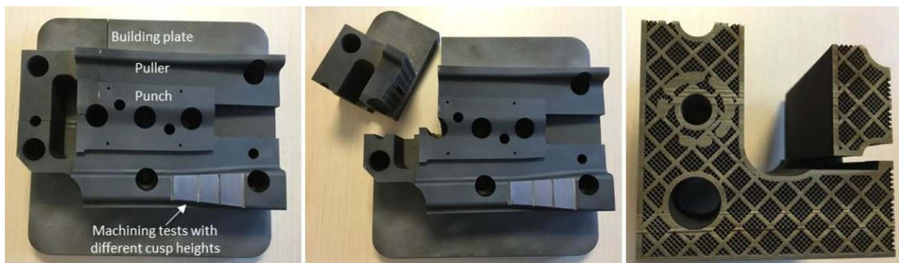
Fig. 13: The 3D-printed puller & punch in the progressive die displayed in Fig. 9. Material = DIN 1.2709. The honeycomb structure has a facade/outer shell thickness of 1.5 mm. Directly after 3D printing: S_a = 5.23 \mu\text{m} and R_a = 4.92 \mu\text{m} . After 3D Printing and milling at cusp height 0.6 \mu\text{m} : S_a = 0.85 \mu\text{m} and R_a = 0.71 \mu\text{m}
