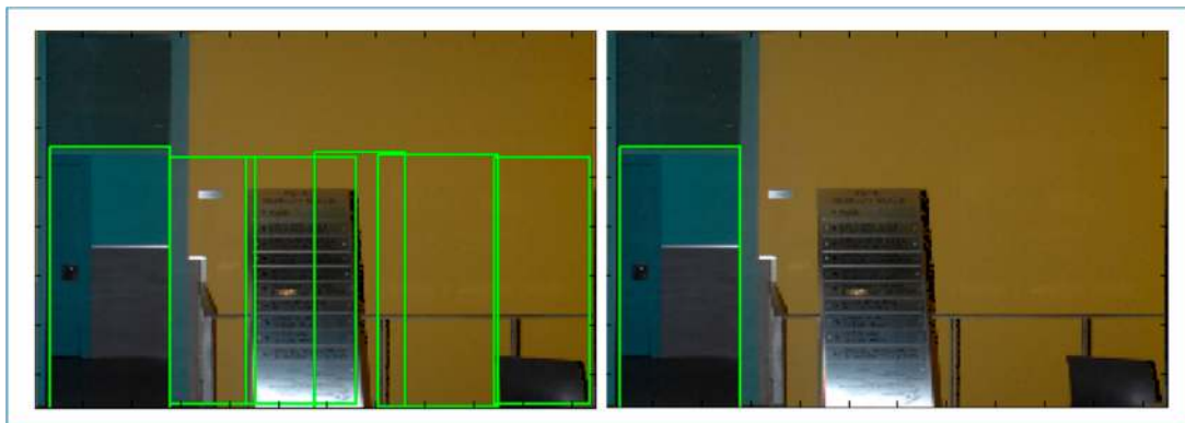
Figure 11. The results of the door extraction are shown before ( left ) and after ( right ) the selection.
