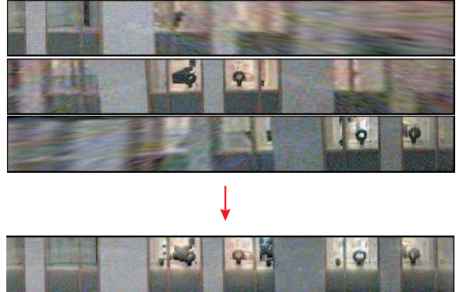
Figure 5: Final textures of walls are generated by blending multiple textures generated from single panoramic images. Shown here are three of ten textures which are fused into a single texture.
