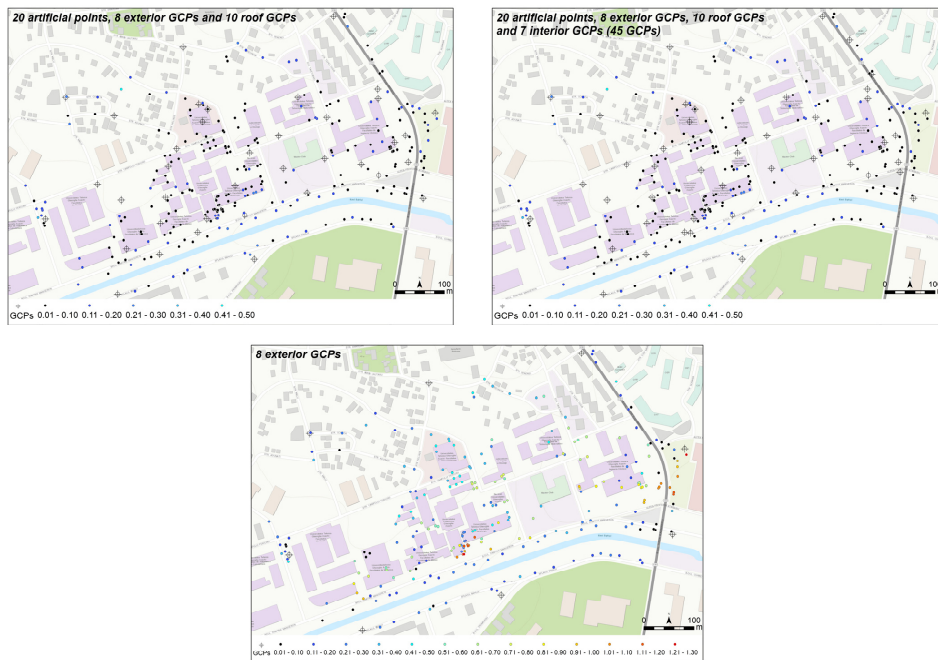
Figure A1. The spatial distribution of GCPs and ChPs and the residuals of 275 ChPs for each scenario.
