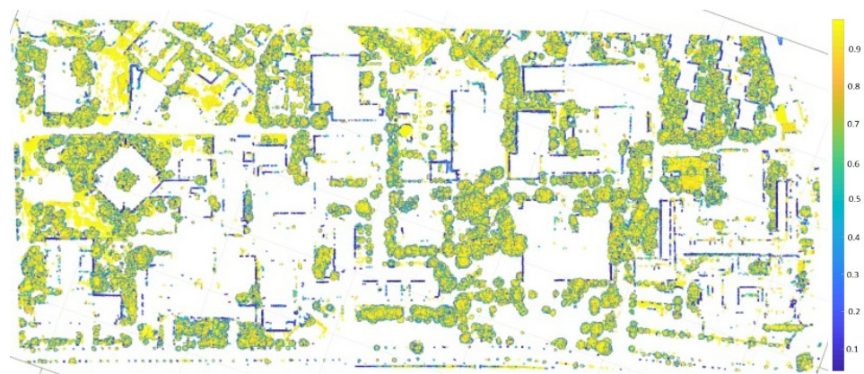
Figure 15. The filtered vegetation points colored by the normal vector component on Z axis.
