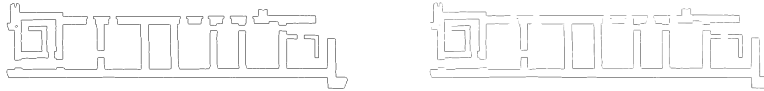
Fig. 4. Edge (left) and straight line (right) images computed from center image in fig. 3.
