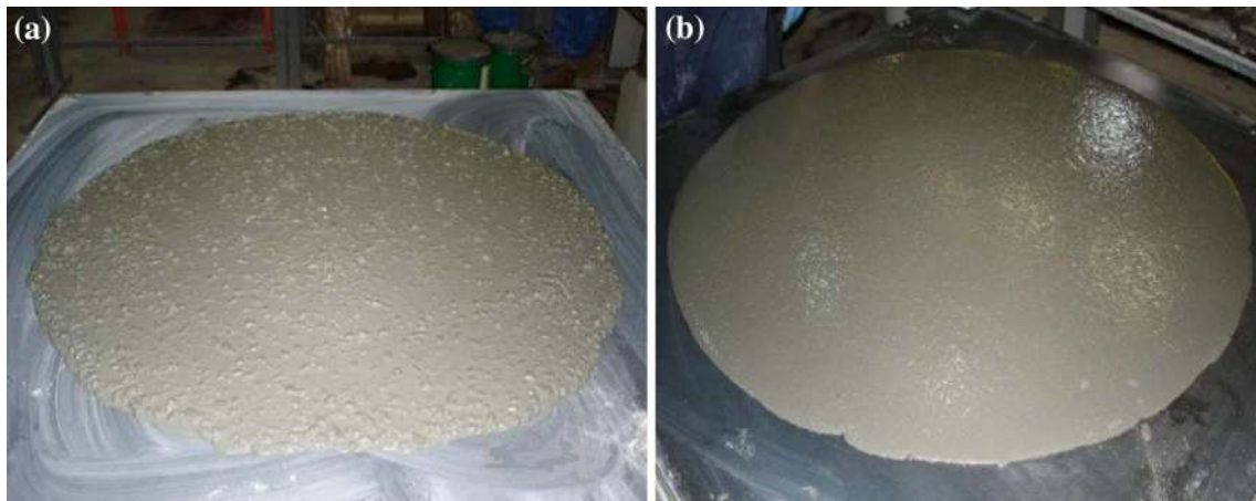
Fig. 2 Horizontal spread of SCC Mix 2 (a) and Mix 4 (b) with fibres
