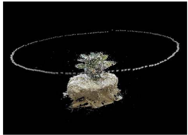
Figure 4. A model constructed from the potted plant sequence showing the sparse 3D point structure and recovered camera positions.
