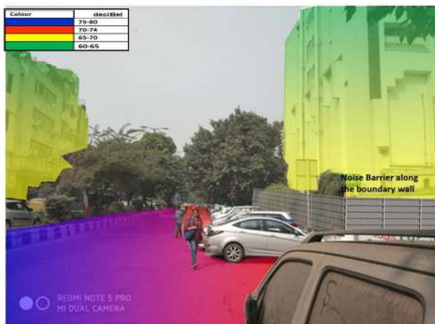
Figure 13: 3D noise mapping of Sukhdev Vihar after installation of noise barrier
