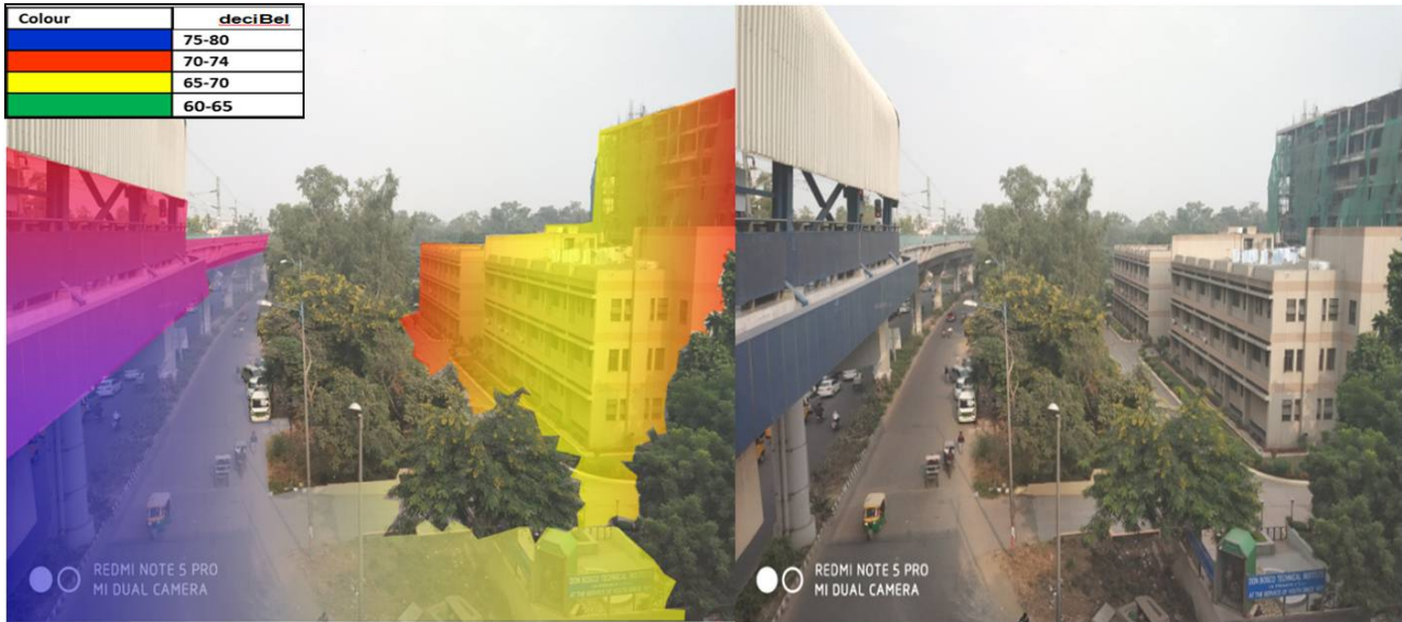
Figure 8: 3D noise mapping of Don Bosco Technical Institute area before installation of noise barrier
