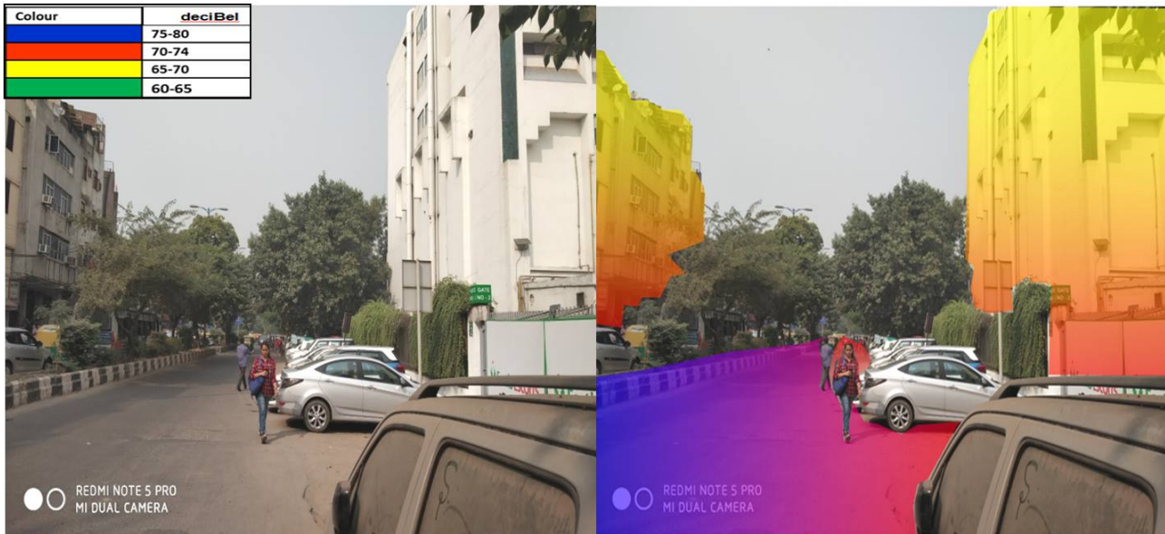
Figure 12: 3D noise mapping of Sukhdev Vihar before installation of noise barrier
