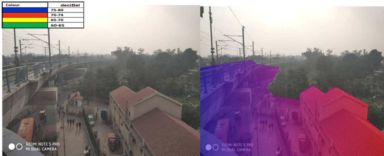
Figure 10: 3D noise mapping of Jamia Millia Islamia (Maktba) before installation of noise barrier
