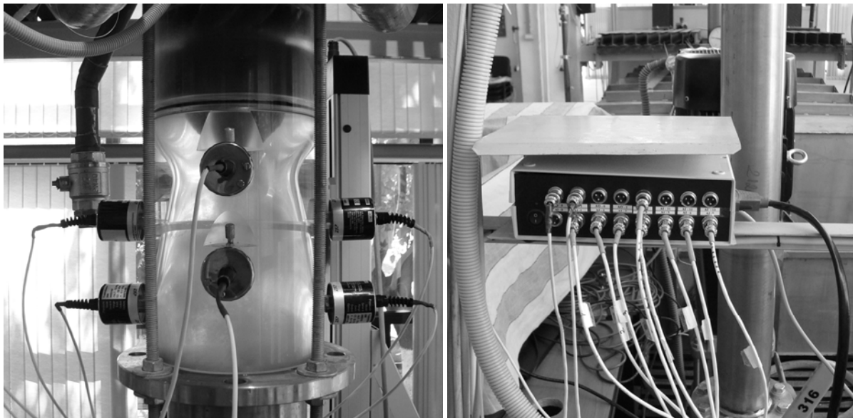
Fig. 3 The unsteady pressure transducers flush mounted on the test section and the integrated data acquisition system.
